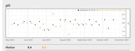
Creek pH is measured using either a YSI probe or a Hach kit that compare a change in water colour. The Environmental Quality Guidelines for Alberta Surface Waters (2018) for exceedance is a pH value outside the range of 6.5 - 9. Data points may overlap.
