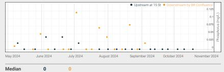
Orthophosphate concentrations are measured with either a LaMotte 1200 Colorimeter or a Hach kit that compare a change in water colour. Data points may overlap.
