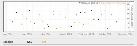
Dissolved oxygen concentrations are measured using either a YSI probe or a Hach kit with a drop-by-drop titration to show a change in water colour until totally clear. Red line indicates the Environmental Quality Guidelines for Alberta Surface Waters (2018) for exceedance is minimum 5 mg/L for instantaneous (short-term) values. Data points may overlap.
