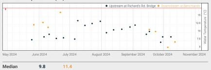
Water temperatures are measured using an Exotech thermometer or YSI probe placed in flowing, shallow water near shore. Red line indicates the Water Quality Objective identified as an ideal value according to the Bow Basin Watershed Management Plan. Values should not exceed a maximum mean of 18°C over a 7-day period. Higher values may cause stress on aquatic life. Data points may overlap.
