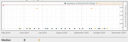
Ammonia nitrogen concentrations are measured by dipping Hach test strips into water and noting the colour change. Red line indicates the Environmental Quality Guidelines for Alberta Surface Waters (2018) for exceedance is maximum 1.0 mg/L at pH 8.0, 10°C. Data points may overlap.
