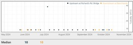
Turbidity is measured by slowly pouring water into a type of graduated cylinder marked with "Nephelometric Turbidity Units" or NTU's or a LaMotte 2020t Turbidity Meter. Data points may overlap.
