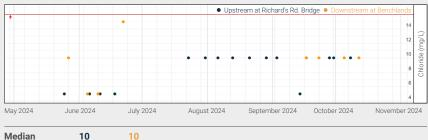
Chloride concentrations are measured using Hach kits with a drop-by-drop titration to show a change in water colour from yellow to orange. Red line indicates the Environmental Quality Guidelines for Alberta Surface Waters (2018) for exceedance is maximum 120 mg/L. Chloride results collected before July 15th, 2024 may have been corrected to account for titrant normality. Data points may overlap.
