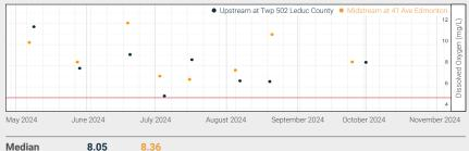
Dissolved oxygen concentrations are measured using either a YSI probe or a Hach kit with a drop-by-drop titration to show a change in water colour until totally clear. Red line indicates the Environmental Quality Guidelines for Alberta Surface Waters (2018) for exceedance is minimum 5 mg/L for instantaneous (short-term) values. Data points may overlap.
