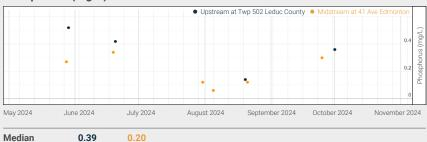
Orthophosphate concentrations are measured with either a LaMotte 1200 Colorimeter or a Hach kit that compare a change in water colour. Data points may overlap.
