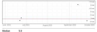
Dissolved oxygen concentrations are measured using either a YSI probe or a Hach kit with a drop-by-drop titration to show a change in water colour until totally clear. Red line indicates the Environmental Quality Guidelines for Alberta Surface Waters (2018) for exceedance is minimum 5 mg/L for instantaneous (short-term) value.
