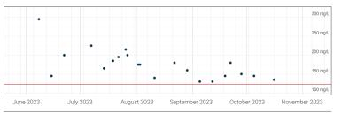
Chloride concentrations are measured using Hach kits with a drop-by-drop titration to show a change in water colour from yellow to orange. Red line indicates the Environmental Quality Guidelines for Alberta Surface Waters (2018) for exceedance is maximum 120 mg/L.
