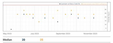
Chloride concentrations are measured using Hach kits with a drop-by-drop titration to show a change in water colour from yellow to orange. Red line indicates the Environmental Quality Guidelines for Alberta Surface Waters (2018) for exceedance is maximum 120 mg/L. Data points may overlap.
