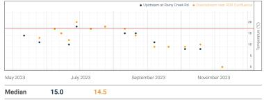
Water temperatures are measured using an Exotech thermometer or YSI probe placed in flowing, shallow water near shore. Red line indicates the Water Quality Objective identified as an ideal value according to the Bow Basin Watershed Management Plan. Values should not exceed a maximum mean of 18°C over a 7-day period. Higher values may cause stress on aquatic life. Data points may overlap.
