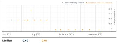
Orthophosphate concentrations are measured with either a LaMotte colorimeter or a Hach kit that compare a change in water colour. Data points may overlap.
