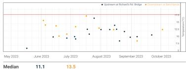
Water temperatures are measured using an Exotech thermometer or YSI probe placed in flowing, shallow water near shore. Red line indicates the Water Quality Objective identified as an ideal value according to the Bow Basin Watershed Management Plan. Values should not exceed a maximum mean of 18°C over a 7-day period. Higher values may cause stress on aquatic life. Data points may overlap.
