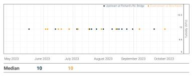
Turbidity is measured by slowly pouring water into a type of graduated cylinder marked with "Nephelometric Turbidity Units" or NTU's. Data points may overlap.
