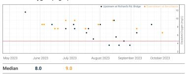
Dissolved oxygen concentrations are measured using either a YSI probe or a Hach kit with a drop-by-drop titration to show a change in water colour until totally clear. Red line indicates the Environmental Quality Guidelines for Alberta Surface Waters (2018) for exceedance is minimum 5 mg/L for instantaneous (short-term) values. Data points may overlap.
