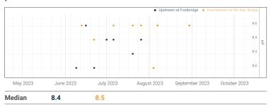
Creek pH is measured using either a YSI probe or a Hach kit that compare a change in water colour. The Environmental Quality Guidelines for Alberta Surface Waters (2018) for exceedance is a pH value outside the range of 6.5 - 9. Data points may overlap.
