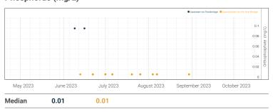
Orthophosphate concentrations are measured with either a LaMotte colorimeter or a Hach kit that compare a change in water colour. Data points may overlap.
