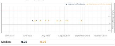
Ammonia nitrogen concentrations are measured by dipping Hach test strips into water and noting the colour change. Red line indicates the Environmental Quality Guidelines for Alberta Surface Waters (2018) for exceedance is maximum 1.0 mg/L at pH 8.0, 10°C. Data points may overlap.
