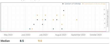
Dissolved oxygen concentrations are measured using either a YSI probe or a Hach kit with a drop-by-drop titration to show a change in water colour until totally clear. Red line indicates the Environmental Quality Guidelines for Alberta Surface Waters (2018) for exceedance is minimum 5 mg/L for instantaneous (short-term) values. Data points may overlap.
