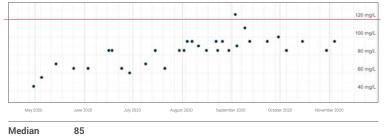
Chloride concentrations are measured using Hach kits with a drop-by-drop titration to show a change in water colour from yellow to orange. Red line indicates the Environmental Quality Guidelines for Alberta Surface Waters (2018) for exceedance is maximum 120 mg/L.
