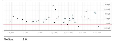
Dissolved oxygen concentrations are measured using either a YSI probe or a Hach kit with a drop-by-drop titration to show a change in water colour until totally clear. Red line indicates the Environmental Quality Guidelines for Alberta Surface Waters (2018) for exceedance is minimum 5 mg/L for instantaneous value.
