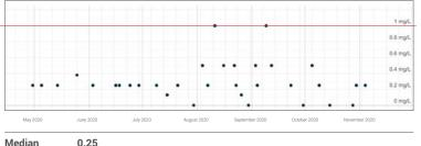
Ammonia nitrogen concentrations are measured by dipping Hach test strips into water and noting the colour change. Red line indicates the Environmental Quality Guidelines for Alberta Surface Waters (2018) for exceedance is maximum 1.0 mg/L at pH 8.0, 10°C.
